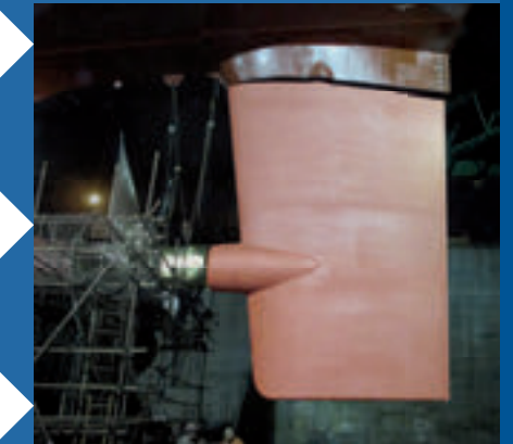
Complete refit with hub cap and a Becker Twist Rudder with bulb
